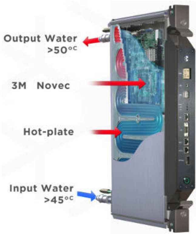
Figure 2. Novec Fluid from 3M is Used in UK-based Iceotope's Data Center Cooling Technology [5]
