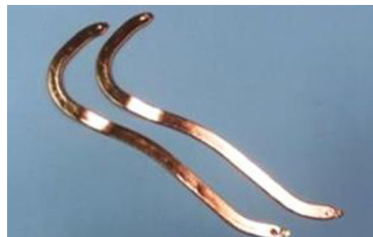
Figure 14. 1.2 mm Thickness Flat Heat Pipe (200 mm Length) [8]
