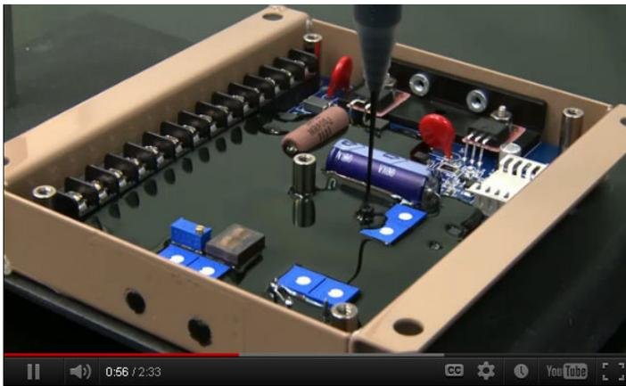
*Figure 2. A Video by Epoxies, Etc. Shows the Application of a Flame Retardant Thermal Epoxy Resin. [6]*
