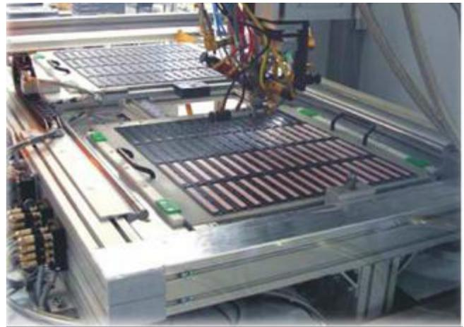
*Figure 3. Some Thermal Compounds Can be Machine Dispensed. [7]*
