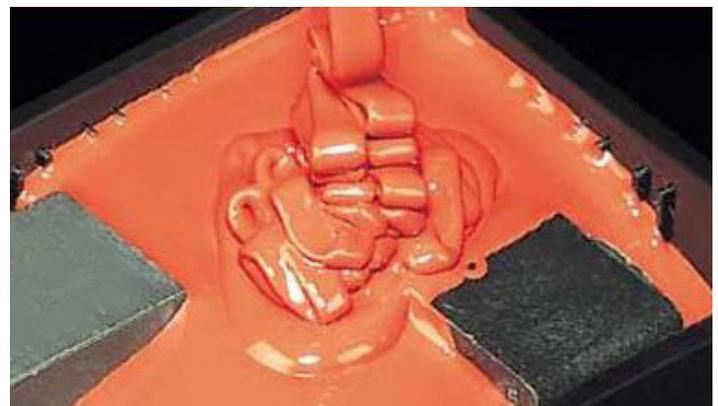
Figure 1. Applying a Thermal Potting Compound.
