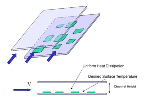
We are trying to find the minimum entrance velocity that can keep the surface temperature below a given maximum value for a known total power dissipation. We are assuming that the power is uniformly distributed over the board.
