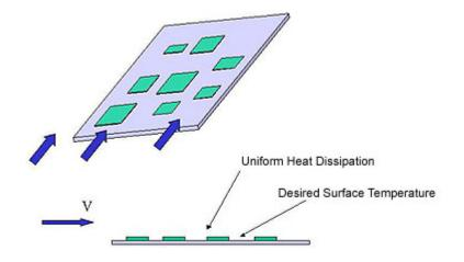
Often we have a maximum surface temperature in mind for a given total power dissipation and we are interested in estimating the average approach velocity of the cooling fluid that can maintain that surface temperature. Since we don't know the velocity, we have to make an assumption about the flow regime, laminar or turbulent. This is an important decision since the correlation that we will use depends on this choice.
