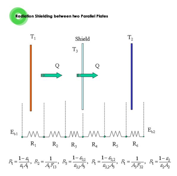
The figure above shows one shield for which the modified heat transfer rate is:
