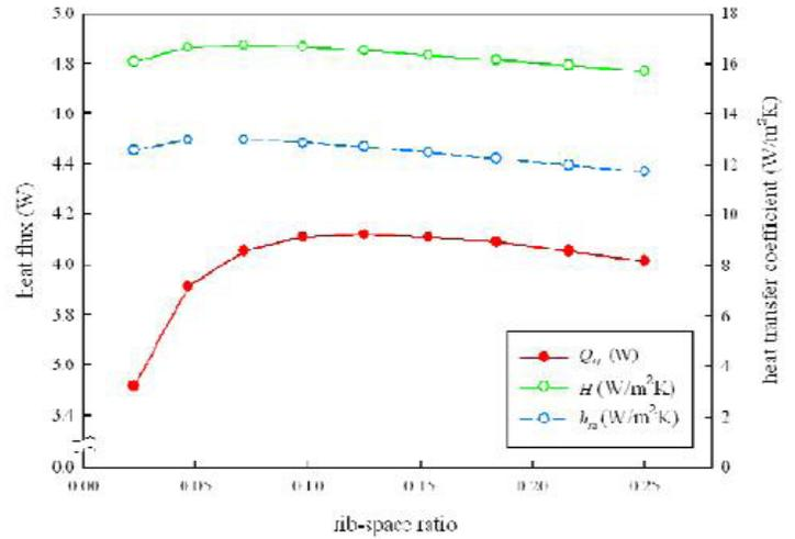
Figure 8. Heat Flux as a Function of Different Rib-Space Ratio [1]
