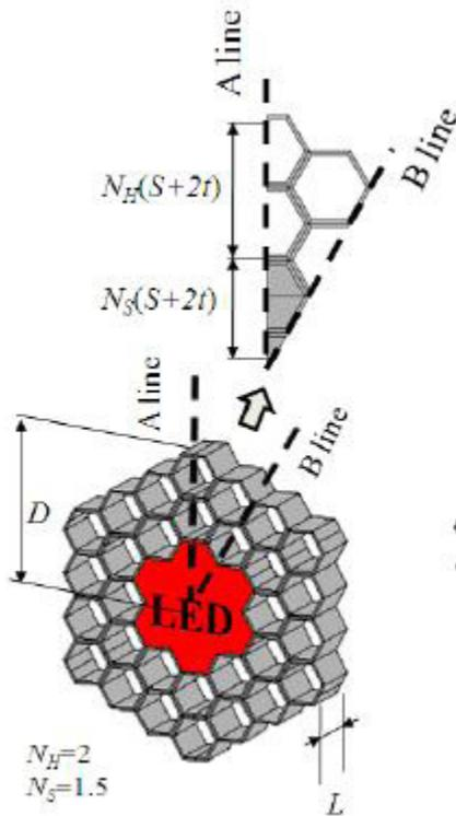
Figure 3. Single Heat Source Honeycomb Heat Sink Model [1]
