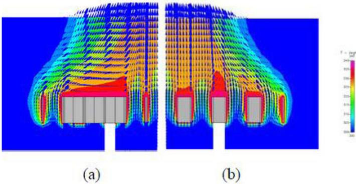
Figure 6. Velocity and Temperature Distribution of the Honeycomb Heat Sink (a) at the Cross Section of the A Line, and (b) at the Cross Section of the B Line [1]
