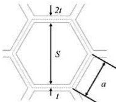
Figure 4. Honeycomb Heat Sink Model Cell Dimension [1]
