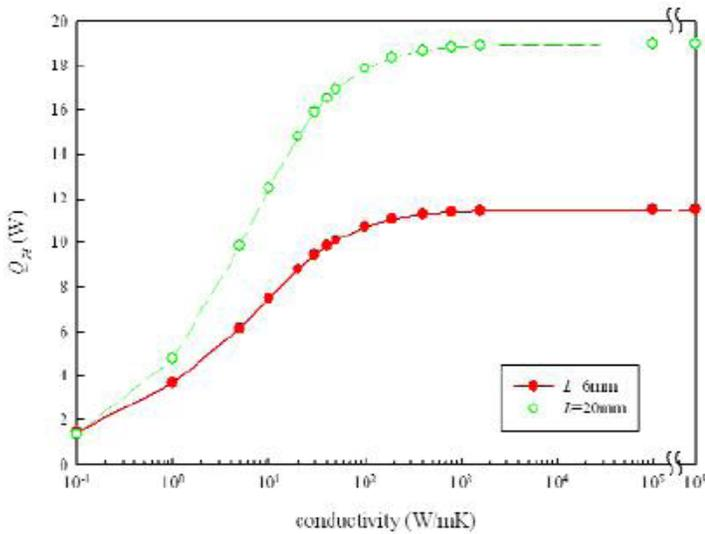
Figure 10. Heat Flux as A Function of Thermal Conductivity [1]
