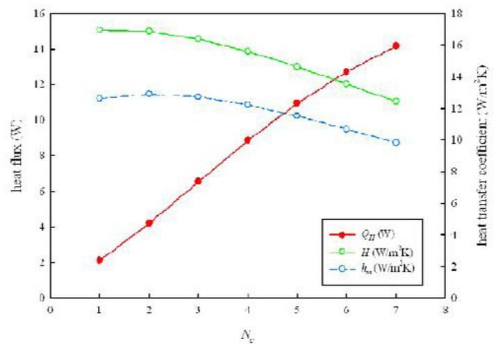
Figure 9. Heat Flux as A Function of Different Number of Cells [1]
