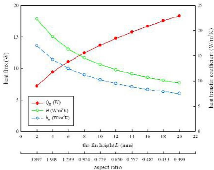
Figure 7. Heat Flux as a Function of Different Cell Aspect Ratio [1]
