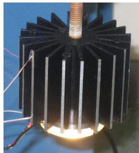
Figure 2. Star LED Heat Sink (Advanced Thermal Solutions, Inc.)
