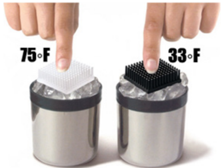
Figure 1. A Demo from Cool Polymers Shows the Performance of a Thermally Conductive Heat Sink vs. a Conventional Plastic Sink [3]
