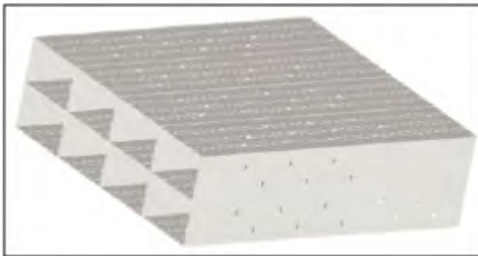
Figure 5. A 2X4 EMI Cage That Was Used in the Flotherm Models for the Forced Convection Setup [2]
