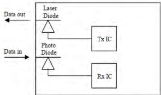
Figure 2. A General Schematic Diagram of a Transceiver [2]
