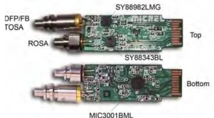
Figure 3. A SFP Module with the Outer Housing Removed to Show the Internal Construction [3]
