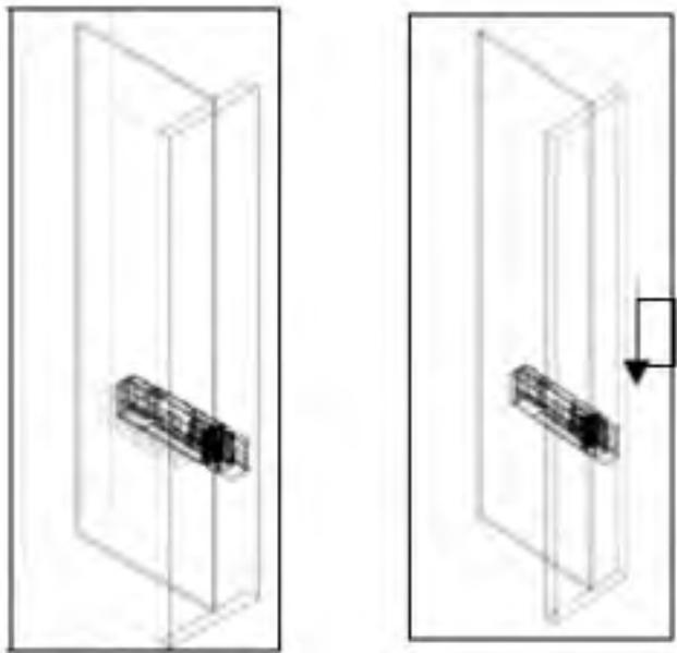
Figure 4. Flotherm Model of an SFP Module With and Without the Heat Sinks in a Natural Convection Setup [2]
