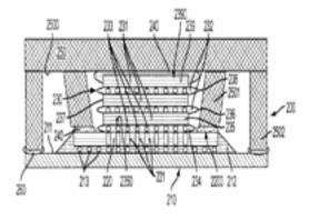
Generally, an electronic package is a hardware component in which active devices, such as logic or memory devices, and passive devices, such as resistors and capacitors, are enclosed. The electronic package performs functions of an electronic system, such as those used inside a mobile phone, a personal computer, a digital music player, etc. Common electronic packages are classified as either flip-chip or wire-bond packages.
