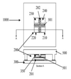
As an example, the second components 210-240 may be segmented into four portions. Here, each of the portions may be disposed proximate to respective corners of the first component 201 with the footprint of the vacated region 202 being defined between the respective footprints of the portions.
