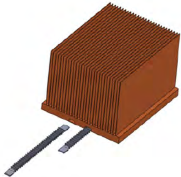
Figure 3. Air-Cooled Heat Sink With Liquid Cooling At The Base [2]
