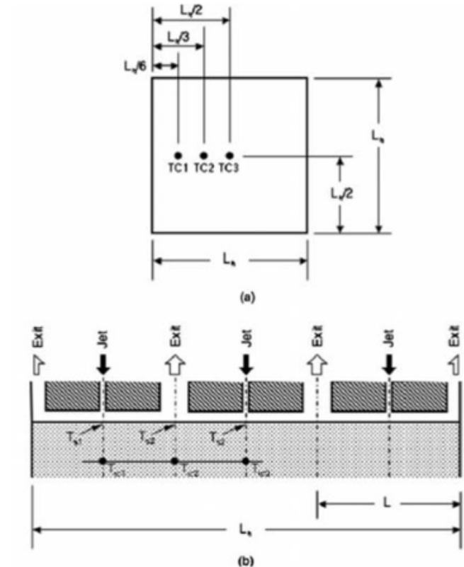
Figure 3. Thermocouple Locations Shown in (a) Top View and (b) Side View of Heater Block [2]
