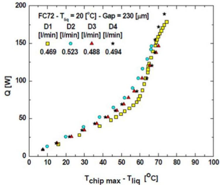
Figure 10. Performance of Different Configurations  $mv=0.5$  l/min and  $T_{liq}=20^{\circ}\text{C}$  [3]
