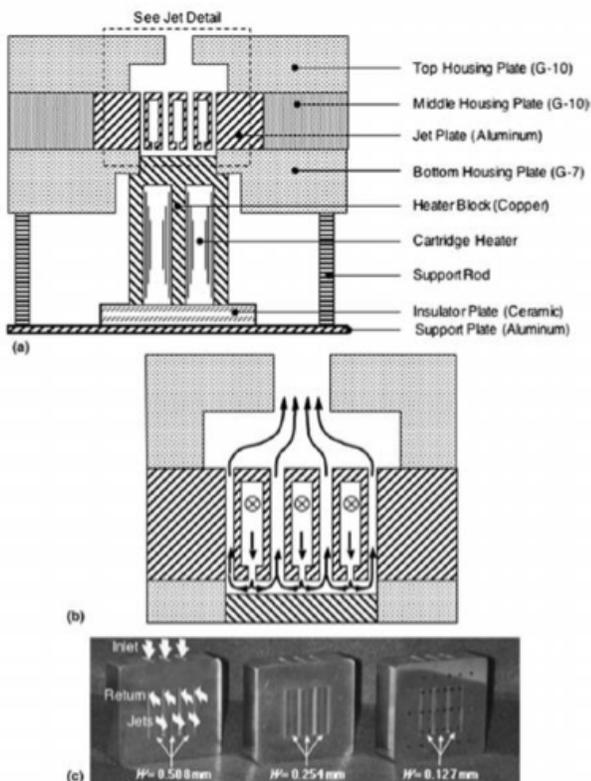
Figure 2. (a) Test Module Schematics (b) Fluid Pattern Inside Test Module (c) Photos of Underside of Jet Plates [2]
