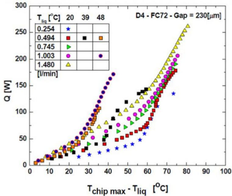
Figure 8. Effect of Different  $T_{liq}$  and Liquid Flow Rate on the Module Performance for Configuration D4 [3]
