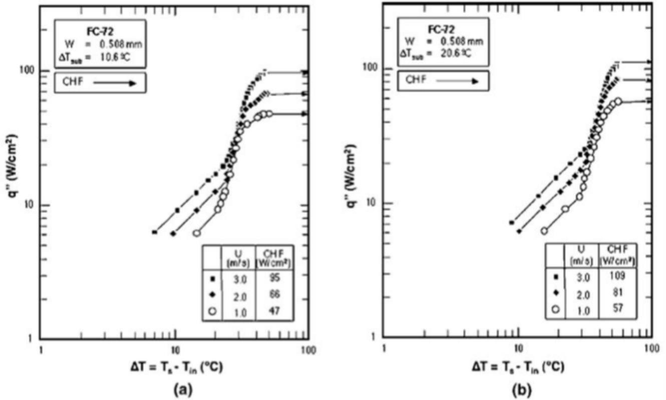
Figure 5. FC-72 boiling Curves for 0.508 mm Jet with (a) 10.6 °C Subcooling and (b) 20.6 °C Subcooling [2]
