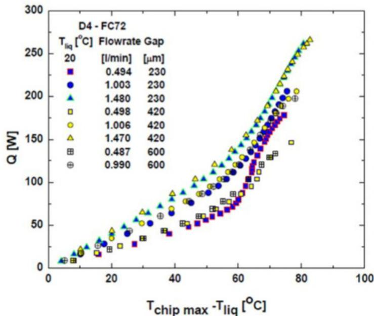
Figure 9. Gap Effect for Configuration D4 and  $T_{liq} = 20^\circ\text{C}$  [3]
