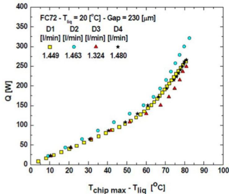
Figure 11. Performance of Different Configurations  $mv=1.5$  l/min and  $T_{liq}=20^{\circ}\text{C}$  [3]
