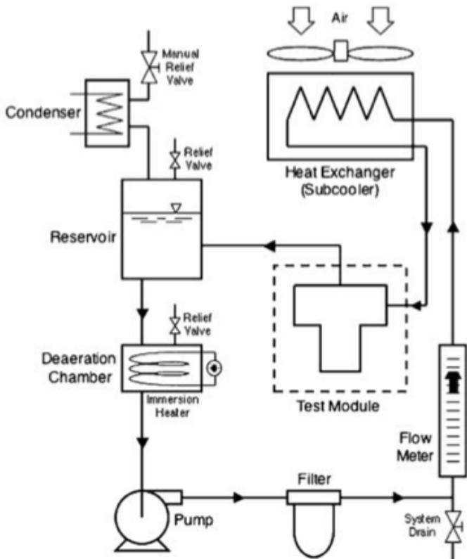
Figure 1. Schematics of Impingement Test Flow Loop [2]
