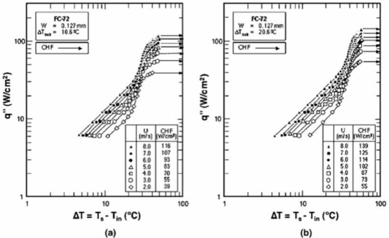
Figure 4. FC-72 Boiling Curves for 0.127 mm Jet with (a) 10.6 °C Subcooling and (b) 20.6 °C Subcooling [2]
