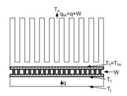
Figure 3. Schematic of a Heat Sink with TEC
