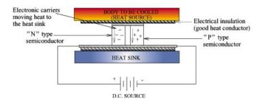
Figure 1. Illustration of a Thermoelectric Module [1]
