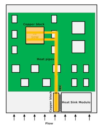
Figure 4. Optimized Heat Sink with TEC Module
