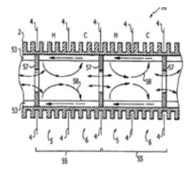
A heat pipe used by the method of this invention by creating alternate adjacent evaporator/condenser pairs along its length can be applied to a variety of applications such as removing heat from electronics or in medical equipment or chemical manufacture. Liquid-to-liquid, liquid-to-air, contact surface-tocontact surface, or air-to-air heat transfer can be accommodated. In this invention, air-to-air heat exchangers for HVAC application will be discussed.
