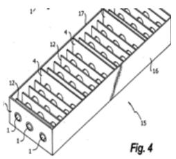
In an alternate embodiment of the heat pipe of this invention, additional torus shaped (like a donut or washer) plugs are added internally to partition each pair or grouping of pairs of heat/cool zones from the adjacent one. The central openings in the plugs allow gas pressures to equalize As the plugs may be rigid and extended to the inside of the heat
