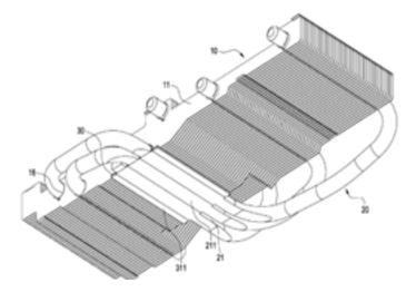
There is a wick structure and working fluid in the heat pipes 20. Heat can be transferred from one end to the other end of the heat pipe 20 by means of phase change of the working fluid. In the shown embodiment, there are three heat pipes 20. Each heat pipe 20 has an evaporation section 21 and one or two condensation sections 22. The evaporation sections 21 are parallely accommodated in the subtroughs 131 of the trough 13.
