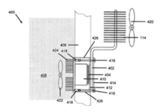
section 106 to evaporation section 102. Evaporation section 102 is connected to a surface from which heat has to be extracted. In an embodiment of the present invention, evaporation section 102 is connected to the thermoelectric device.
