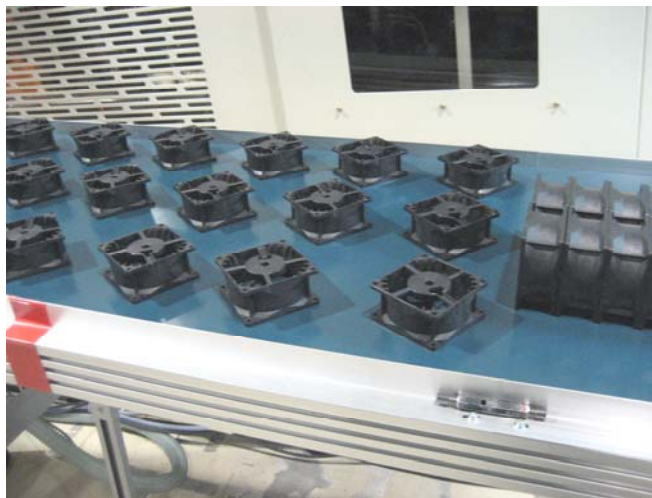
Figure 3. Fan frames being arranged after injection molding
